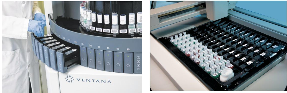
Figure 23. Two example of staining machines used in pathology laboratories. Benchmark Ultra (left) and Autostainer (right).
